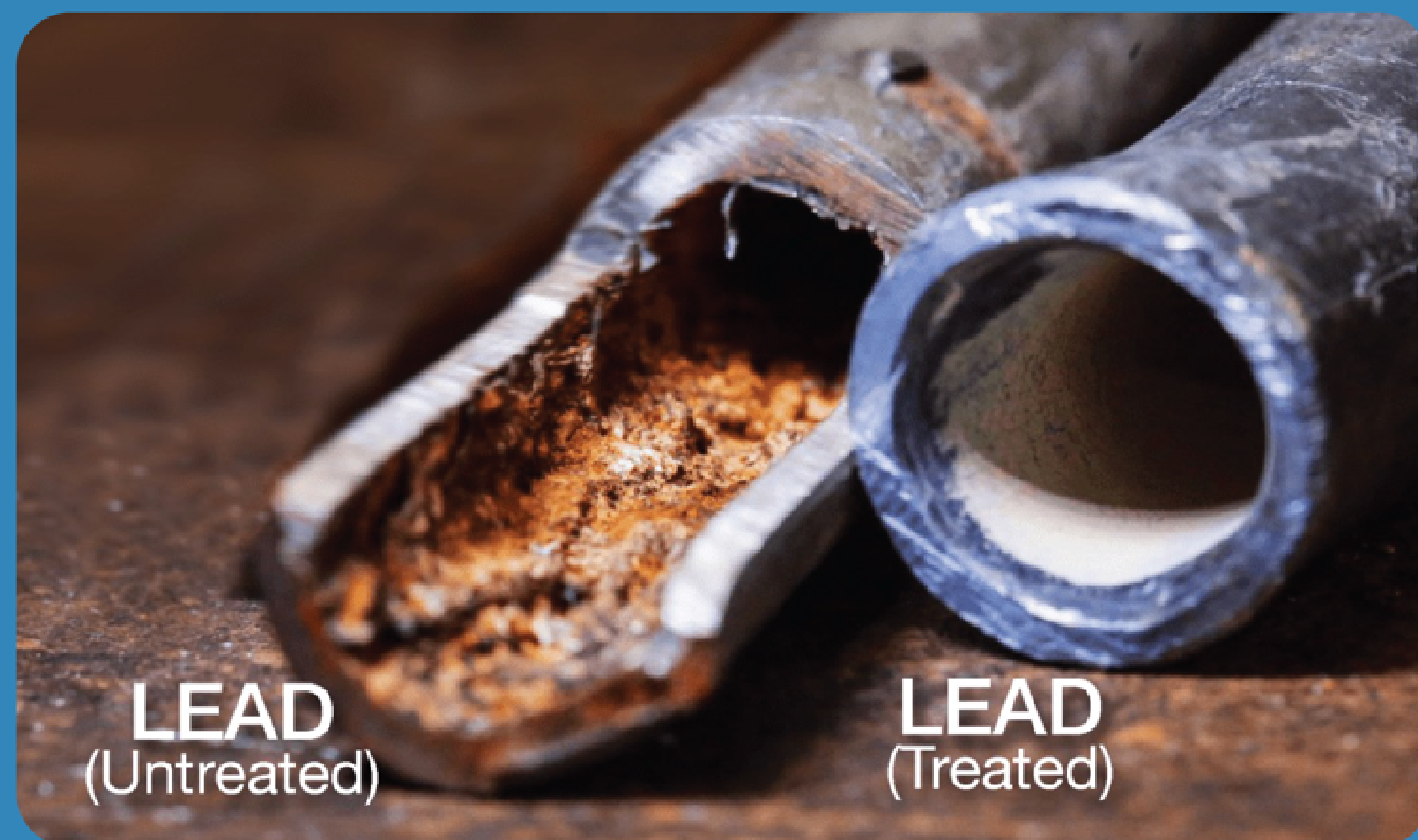
Figure 1. Untreated (Left) vs. Treated (Right) Lead Pipes
